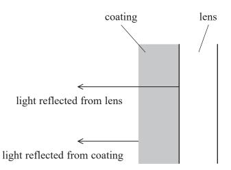
When a single-layer coating is used, the coating thickness is chosen to eliminate reflections for green light, which is in the middle of the visible spectrum.
