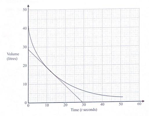
Using the graph, work out an estimate for the rate at which the water is flowing out of the container when t = 12
