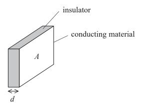
The capacitor has a capacitance  $0.1\,\mu\text{F}$  and is charged to a p.d. of  $100\,\text{V}$  by connecting it to an electrical supply.
