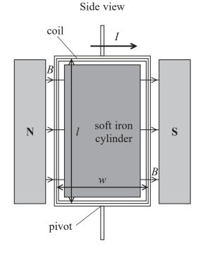
The fixed soft iron cylinder and magnets produce a uniform magnetic field of magnetic flux density B. The coil is able to rotate within this magnetic field. The coil has width w and length l. There is a current l in the coil in the direction shown in the side view diagram.
