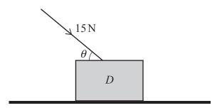
A block D of weight 50 N lies at rest in equilibrium on a fixed rough horizontal surface. A force of magnitude 15 N is applied to D at an angle  $\theta$  to the horizontal (see diagram).
