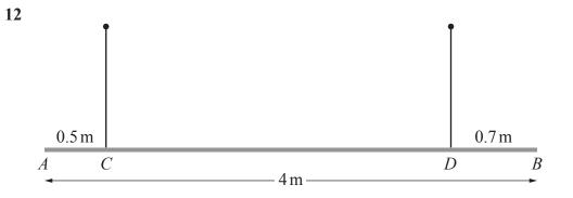
A beam, AB, has length 4 m and mass 20 kg. The beam is suspended horizontally by two vertical ropes. One rope is attached to the beam at C, where AC = 0.5 m. The other rope is attached to the beam at D, where DB = 0.7 m (see diagram).
