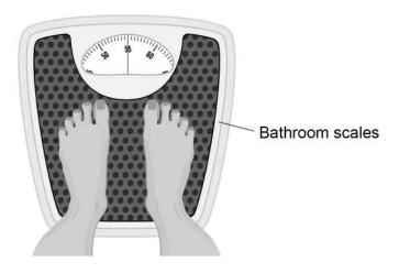
The person exerts a downward force on the scales and the scales exert an upward force on the person.
