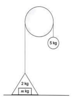
The mechanism is released from rest, and the container begins to move upwards with acceleration  $a\,\mathrm{m}\,\mathrm{s}^{-2}$
