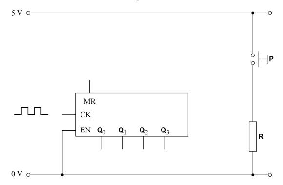
The counter resets when the master reset pin MR receives a logic 1
