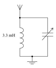
**0 2 . 1** The circuit is tuned to receive a radio station transmitting at a frequency of 1053 kHz.
