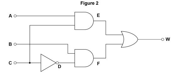
Write the Boolean algebra expression for output **W** in terms of the inputs **A**, **B** and **C**. The expression must contain only the four logic gate operations shown in **Figure 2**. [2 marks]
