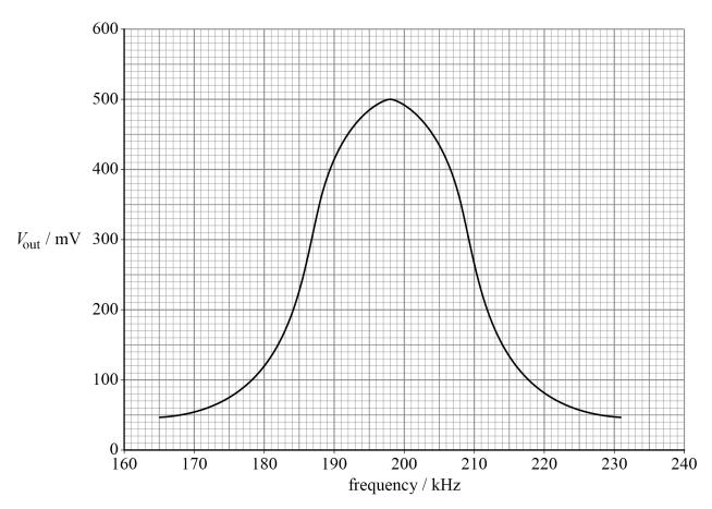
Determine the bandwidth of the filter circuit.
