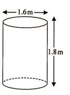
Area of top and bottom =  $2 \times \pi \times 0.8^2 = 1.28\pi$ Area of curved rectangle =  $1.8 \times 1.6 \pi = 2.88\pi$ Total area of one tank =  $4.08\pi m^{2}$ . Area of 3 tanks =  $12.24\pi m^{2} = 38.45m^{2}$   $7 \times 5m^{2} = 35m^{2}$  of paint. 38.45735
