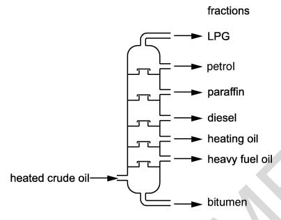
(a) Crude oil contains a mixture of hydrocarbons that boil at different temperatures.
