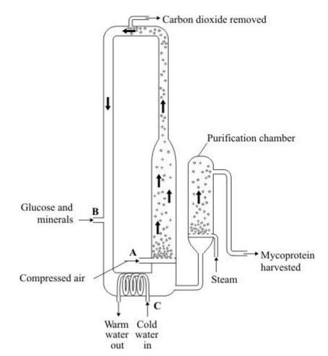
(a) Bubbles of air enter the fermenter at A.
