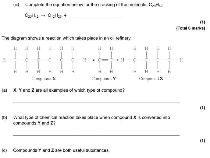
Compound Y is unsaturated. Compound Z is saturated.
