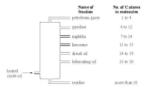
(i) Explain, as fully as you can, how fractional distillation works.
