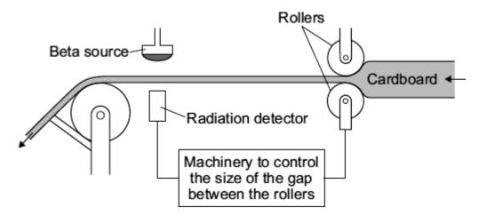
The cardboard passes through a narrow gap between a beta radiation source and a radiation detector.
