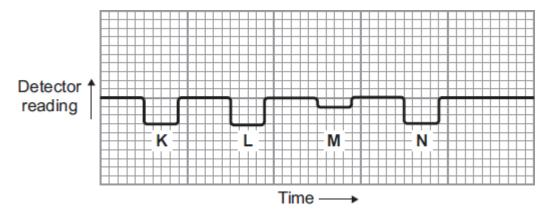
Which part of the chart,  $\mathbf{K}$ ,  $\mathbf{L}$ ,  $\mathbf{M}$  or  $\mathbf{N}$ , shows that an empty box is passing between the beta source and the detector?
