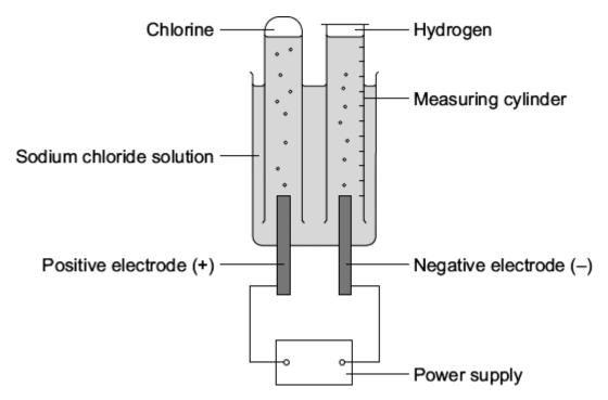
The student measured the volume of hydrogen gas produced in ten minutes.
