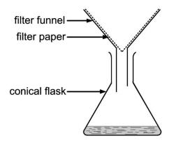
The equipment shown in the diagram can be used to separate a mixture of sand and water but **cannot** be used to separate salt from a solution in water.
