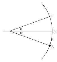
(e) Using this result, demonstrate that the acceleration of a mass moving around a circle with a radius of r at a speed of v is  $a = \frac{v^2}{r}$ .
