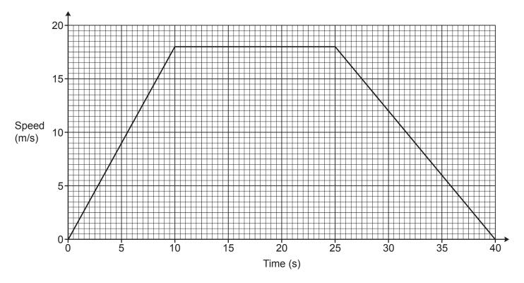
(a) Write down the acceleration of the car between 10 seconds and 25 seconds.
