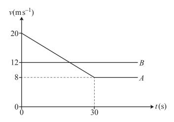
The diagram shows a velocity-time graph representing the motion of two cars A and B which are both travelling along a horizontal straight road. At time t = 0, car B, which is travelling with constant speed  $12 \,\mathrm{m\,s}^{-1}$ , is overtaken by car A which has initial speed  $20 \,\mathrm{m\,s}^{-1}$ .
